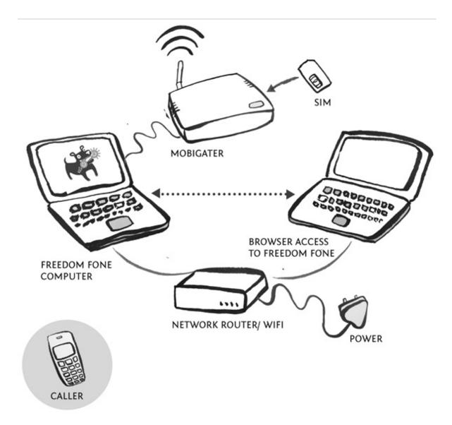
The diagram above shows how to connect to the MobiGater.
