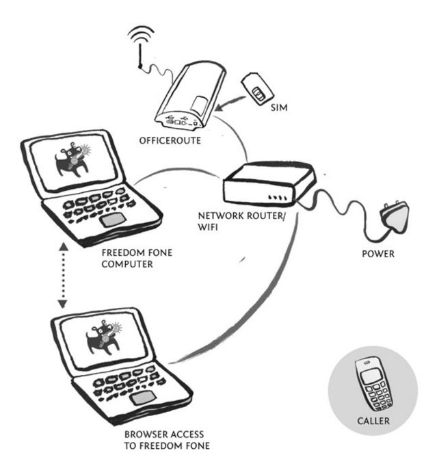
The diagram above shows how you would connect a computer running Freedom Fone to an OfficeRoute. Note that you can also connect the OfficeRoute directly to your Freedom Fone computer using a crossover cable.
